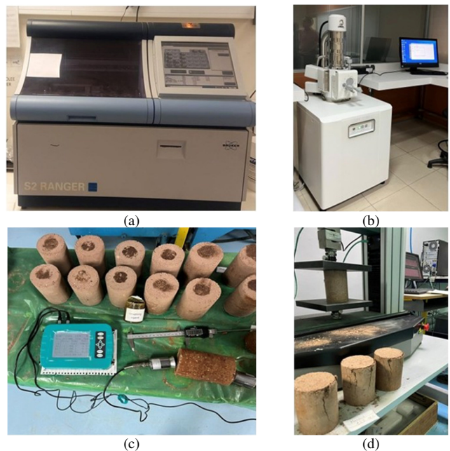
Fig. 2. Experimental testing equipment used in the study: (a) XRF analysis, (b) SEM observation, (c) UPV measurement, and (d) compressive strength test.
