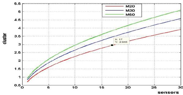
Fig. 2. Optimum number of clusters versus sensors and network size.
