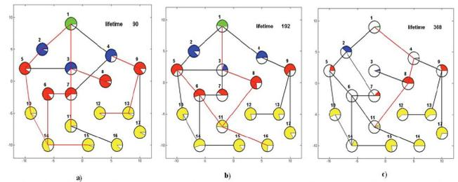
Fig. 5. WSN lifetime using a node energy level threshold value for routing change.
