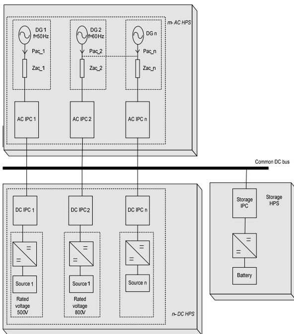
Fig. 1. Intertied hybrid system topology
