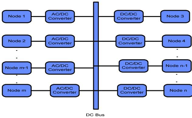
Fig. 4. Interconnection of IPC in intertied hybrid system
