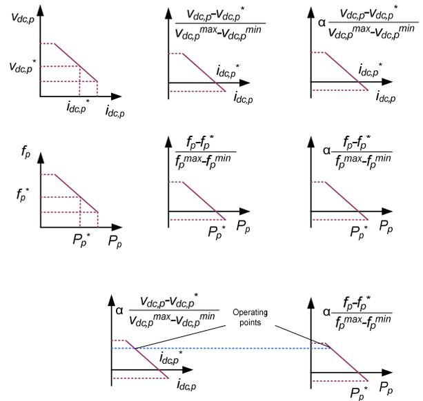
Fig. 5. Corrections for Coordinated Power Control
