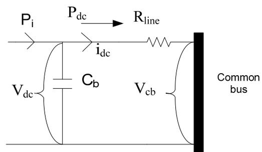
Fig. 2. Circuit simplification for proposed droop control
