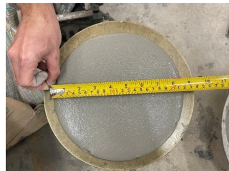
Fig. 2. The flowability of cement plaster containing \text{BaSO}_4 .
