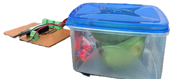
Fig. 3. Fruit box with embedded sensors.
