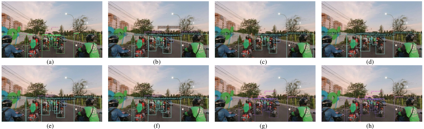
Fig. 2. Visualization of (a) ground truth bounding boxes, as well as detection results of (b) Faster R-CNN Resnet50 input size 800, (c) SSD VGG16 input size 640, (d) SSD-Lite MobileNetV3-large input size 320, (e) RetinaNet ResNet50 input size 800, (f) FCOS ResNet50 input size 800, (g) DETR ResNet50 input size 480, and (h) Conditional DETR ResNet50 input size 480.
