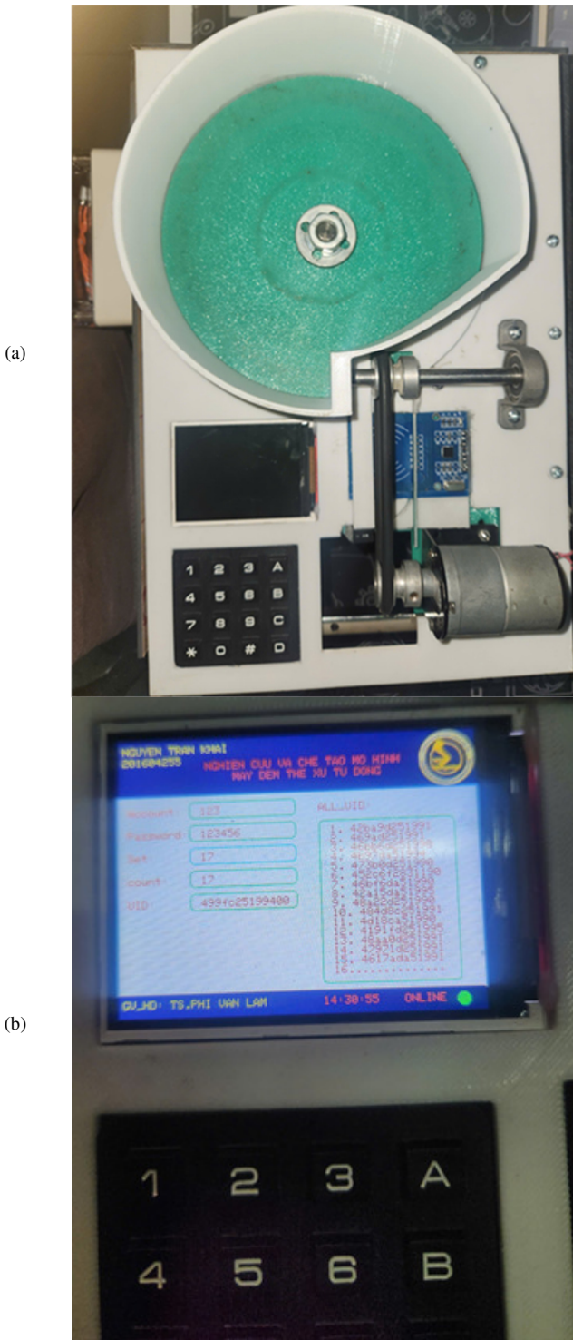
Fig.8. Experimental prototype of the IoT-enabled automatic token counting device: (a) top view, (b) display screen.
