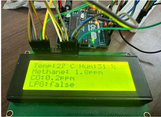
Fig. 10. LCD Displaying with the measured values of methane, CO, and LPG levels at the top of the borewell system.
