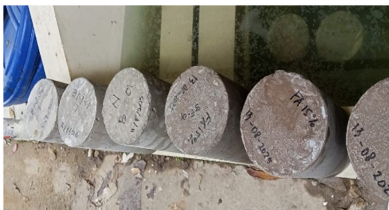
Fig. 2. Concrete after immersion in normal water.
