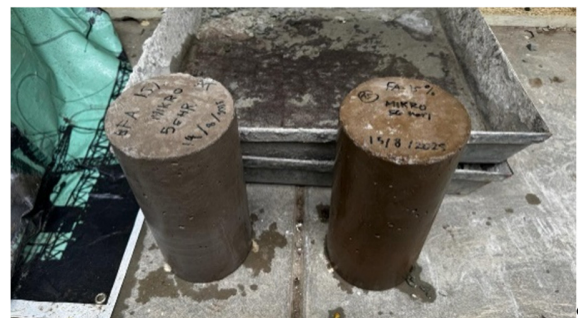
Fig. 3. Concrete after immersion in sulfuric acid water and acid mine water.
