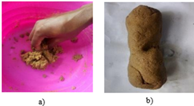
Fig. 5. (a) Rice husk + GA + water mixing using the hands and (b) rice husk + GA paste ready for extrusion.
