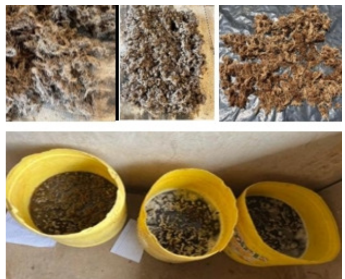
Fig. 4. Fiber cutting, treatment, and drying.
