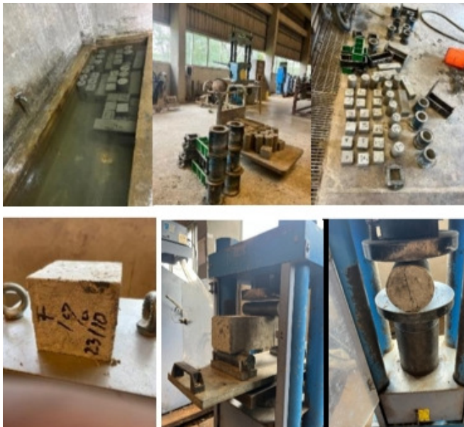
Fig. 6. Concrete curing and testing.
