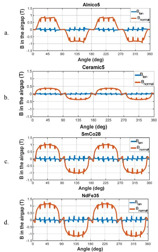
Fig. 8. Comparison of B components in the air gap for different magnet materials using the reference magnet embrace 0.833
