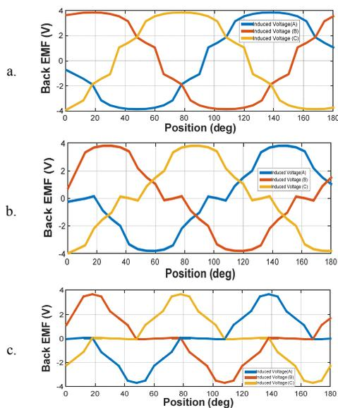
Fig. 14. Comparison of back EMF for different magnet embraces
