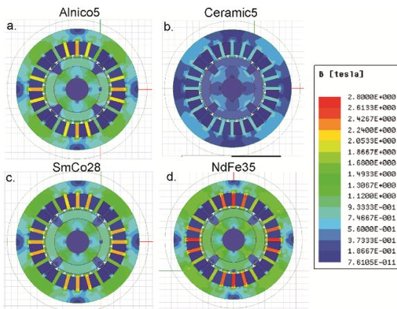
Fig. 6. The distribution of B in the machine for different magnet materials using the reference magnet embrace 0.833
