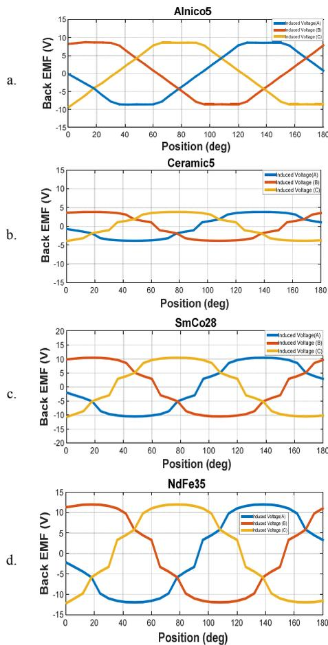
Fig. 10. Comparison of back EMF for different magnet materials using the reference magnet embrace 0.833
