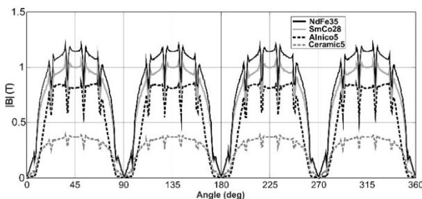
Fig. 7. Comparison of |B| in the airgap for different magnet materials using the reference magnet embrace 0.833
