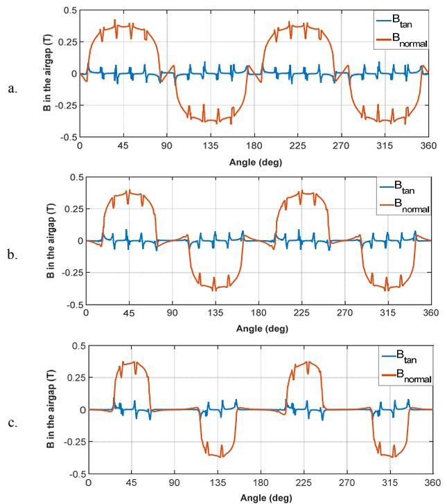
Fig. 12. Comparison of  $B$  components in the air gap for magnet embraces a. 0.833, b. 0.625 c. 0.416 of Ceramic5 magnet
