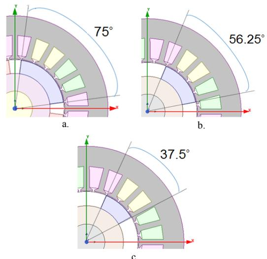
Fig. 5. The BLDC geometries of different magnet embraces investigated in this study: a. the reference magnet embrace 0.833, b. magnet embrace 0.625, and c. magnet embrace 0.416.
