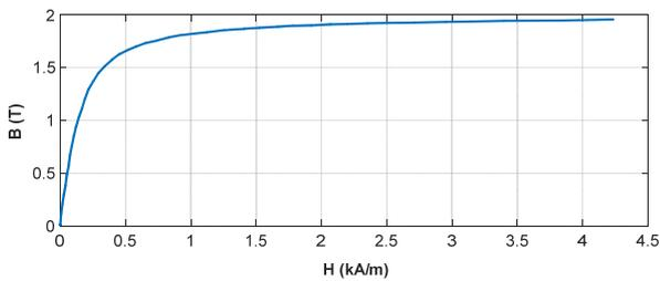
Fig. 2. The B-H curve of the ferromagnetic material used for the stator and rotor core
