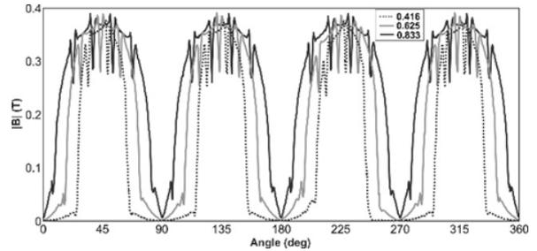
Fig. 11. Comparison of  $|B|$  in the air gap for Ceramic5 magnet material using three different magnet embraces
