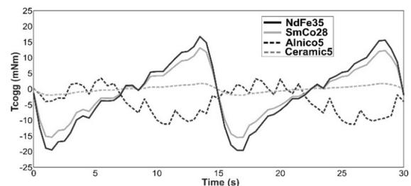
Fig. 9. Comparison of the cogging torque for different magnet materials using the reference magnet embrace 0.833
