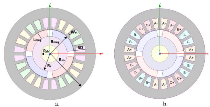
Fig. 1. a. BLDC motor geometry, b. Assignment of the excitations to the coils
