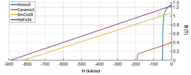
Fig. 3. B-H curves of permanent magnet materials
