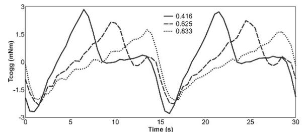
Fig. 13. Comparison of  $T_{cog}$  for different magnet embraces
