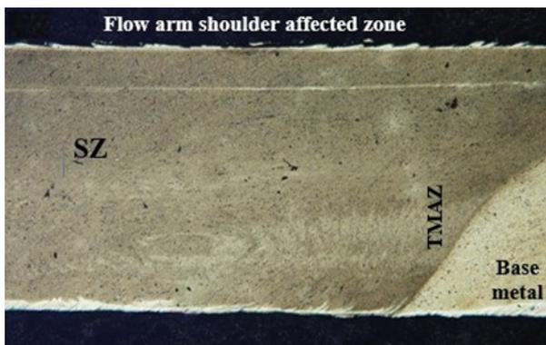
Fig. 4. A micrograph of the joints at 35 mm/min traverse speed and 900 rpm rotational speed.
