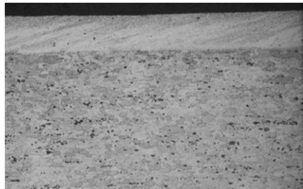
Fig. 2. Optical microstructure of the base metal.
