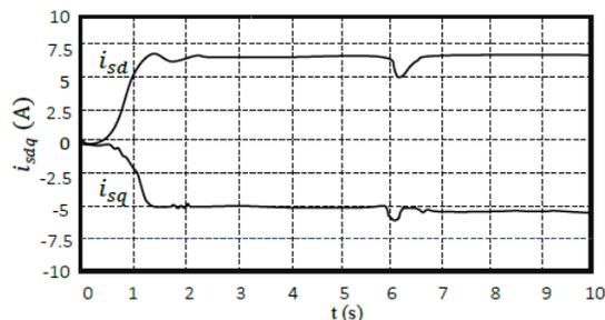
Fig. 11. Changes in the d and q components of the stator current
