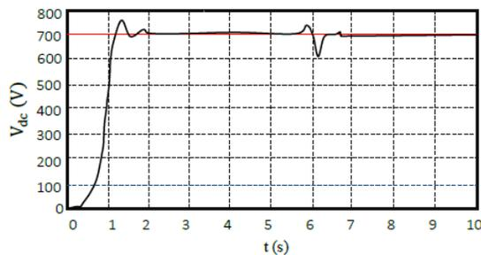
Fig. 10. The generated DC voltage
