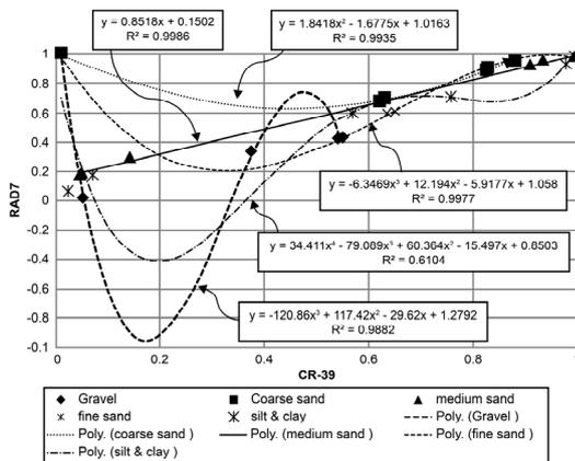
Fig. 8. Relationship between R<sup>2</sup> values for the correlations determined using Cr-39 and Rad7 techniques
