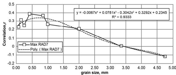
Fig. 3. Grain size vs. its correlation with radon content according to cumulative % passing
