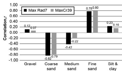
Fig. 6. Correlation between radon content and various grain size fractions for both CR-39 and Rad 7 techniques
