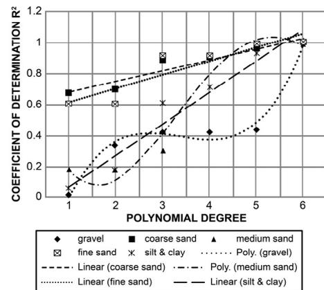
Fig. 5. R<sup>2</sup> values for different degrees of the polynomial function and different grain sizes
