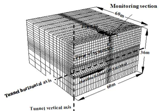
Fig. 2. Three-dimensional finite element mesh
