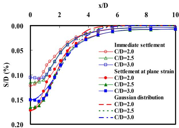
Fig. 4. Transverse settlement at monitoring section due to tunnelling
