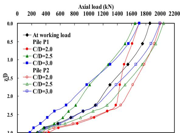
Fig. 7. Axial load changes in P1 and P2 due to tunnelling
