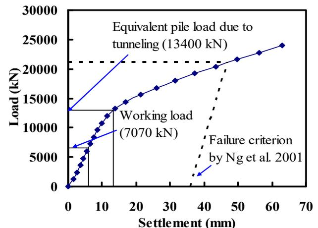
Fig. 3. Load settlement curve of simulated pile group load test
