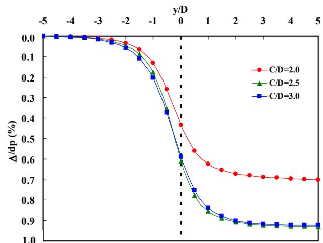
Fig. 5. Pile cap settlement due to tunnel advancement
