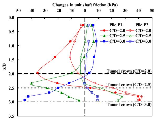
Fig. 6. Changes in unit shaft friction due to tunnelling
