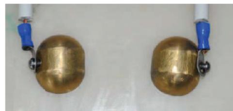
Fig. 2. The electrodes of the experimental setup. Their distance is 2.5 cm.
