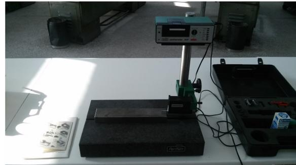
Fig. 3. Perthometer M4P. The measurements took place at the Machine Tools and Quality Control Laboratory of the Technological Educational Institute of Eastern Macedonia and Thrace.
