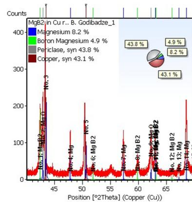
Fig. 7. The diffraction picture of HEC Mg-2B composite powders after consolidation at  $940^\circ C$  in copper container.
