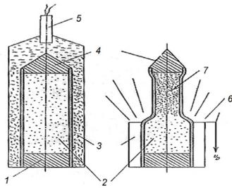
Fig. 1. The procedure of preliminary densification of Mg-2B blend powders: 1. Bottom plug of copper tube. 2. Precursor powders. 3. Explosive powder. 4. Upper plug of steel tube. 5. Electric detonator. 6. Products of detonation. 7. Consolidated powders.
