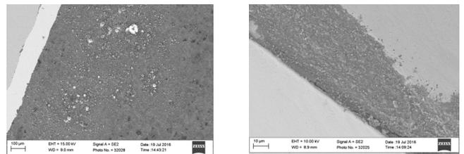
Fig. 6. The macrostructure of HEC Mg-2B precursors at  $940^\circ C$  in copper container with application of intermediate Tantalum layer.
