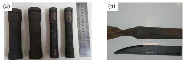
Fig. 4. The billets from Mg-2B blend powders after consolidation with intensity of loading under 10 GPa: a) first stage pre-densification by shock waves at room temperatures, b) consolidation of the same billets at  $1000^{\circ}\text{C}$  with intensity of loading under 5 GPa.
