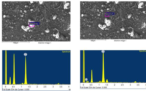
Fig. 10. The microstructures of HEC Mg-2B composites and their correspondent spectral analyses with element identification obtained at 940°C with application of intermediate Ta layer. The intensity of loading onto the container's wall was around 5 GPa.
