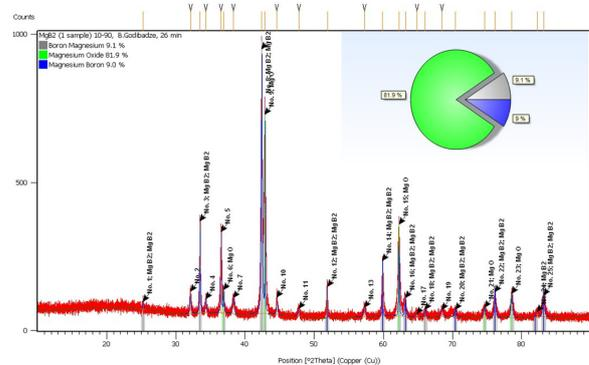
Fig. 8. The diffraction picture of HEC Mg-2B composite powders obtained at  $940^\circ C$  in copper container with application of protecting intermediate Tantalum layer.
