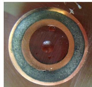
Fig. 12. View of cross-section of hybrid Cu- $MgB_2$ -Cu superconducting tube.
