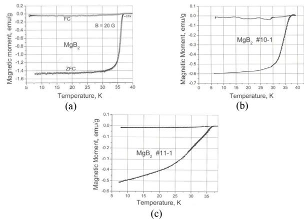
Fig. 11. Magnetic moment temperature dependence measurements in zero-field-cooled (ZFC) and field-cooled (FC) modes, showing the superconducting transition depending on container material and type of boron precursors. a) HEC in steel container at 1000°C. b) HEC in Cu container with  $^{10}B$  isotope at 940°C. c) HEC in Cu container with  $^{11}B$  isotope at 940°C.
