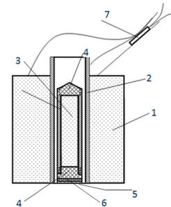
Fig. 3. Experimental set up for HEC of cylindrical billets explosive charge at the bottom according to the general view of HEC device (Figure 1).
