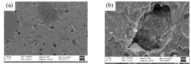
Fig. 5. The microstructure of HEC Mg-2B blend powders after two stage shock wave loading in copper container at  $940^\circ C$  with loading intensity of 5GP: a) central part b) edge.
