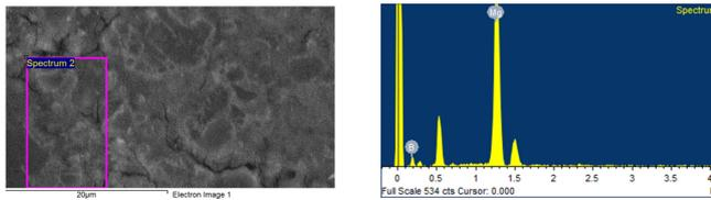
Fig. 9. The macrostructure of HEC Mg-2B precursors near to the edge obtained at 940°C using intermediate Ta layer. As it's seen from spectral analysis and atom distribution there diffusion of copper atoms into the HEC Mg-2B precursors is fully prevented.
