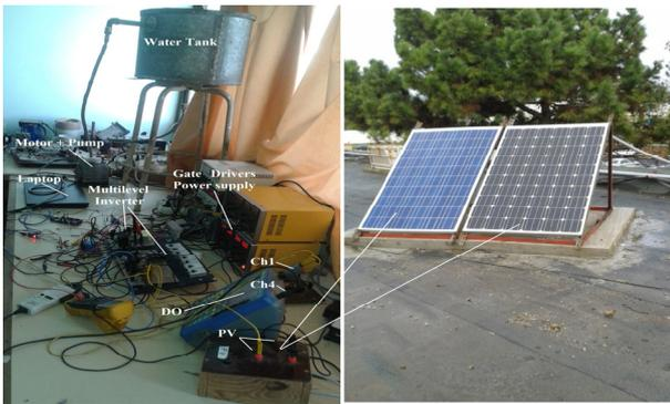
Fig. 18. The two solar panels installed at the laboratory roof with the full PV system.
