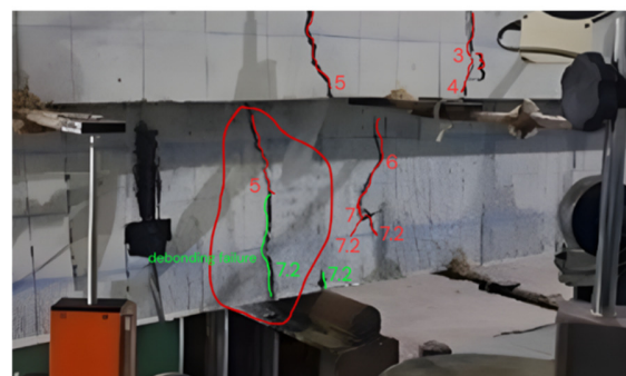
Fig. 7. Test documentation for specimen side-bonded.
