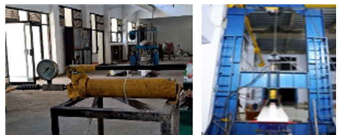
Fig. 1. Hydraulic jack and loading frame.
