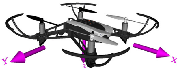
Fig. 4. Coordinate and force CS on a quadcopter.
