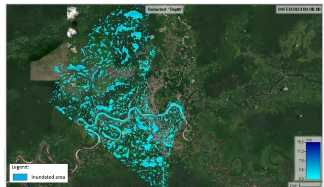
Fig. 10. Extent of inundated area before restoration in Oxbow Lakes (Sinau, Jaras, and Selanyut) using HEC-RAS modeling.
