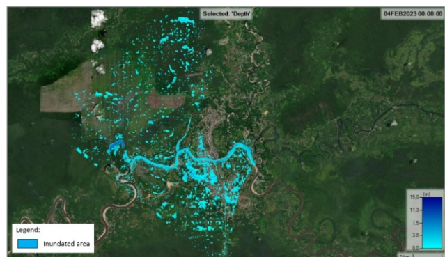
Fig. 11. Extent of inundated area after restoration in oxbow lakes (Sinau, Jaras, and Selanyut) using HEC-RAS modeling.
