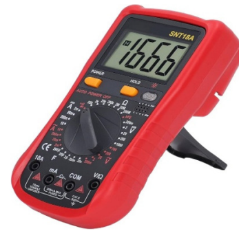
Fig. 6. The digital multimeter, with a DC voltage reading range of 0–1000 V with an accuracy of \pm 0.5\% .
