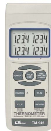
Fig. 7. Four channels thermometer TM-946 with a measurement range of -50°C to +1300°C.
