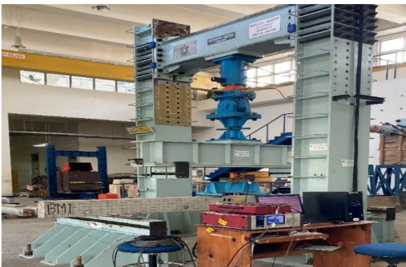
Fig. 4. A UTM is used for a two-point static loading test.
