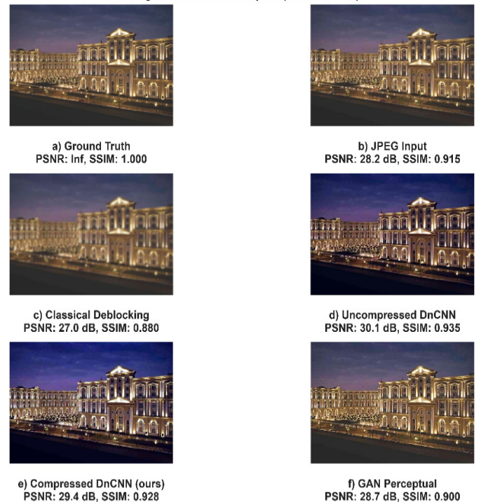
Fig. 4. Full-image restoration examples for an image compressed at JPEG quality Q = 30 . (a) Ground truth, (b) JPEG-compressed input, (c) classical deblocking, (d) uncompressed DnCNN, (e) compressed DnCNN (proposed), (f) GAN-based perceptual model.
