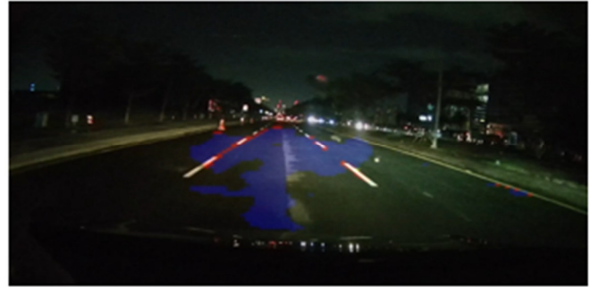
Fig. 5. Example of failure cases under rainy and nighttime conditions showing partial segmentation loss caused by low illumination, glare, and reflective road surfaces.
