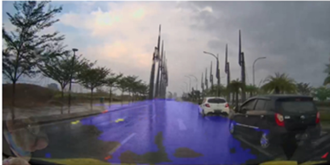
Fig. 5. Example of failure cases under rainy and nighttime conditions showing partial segmentation loss caused by low illumination, glare, and reflective road surfaces.
