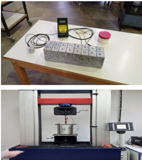
Fig. 4. Pull-out bond test setup and UPV test.
