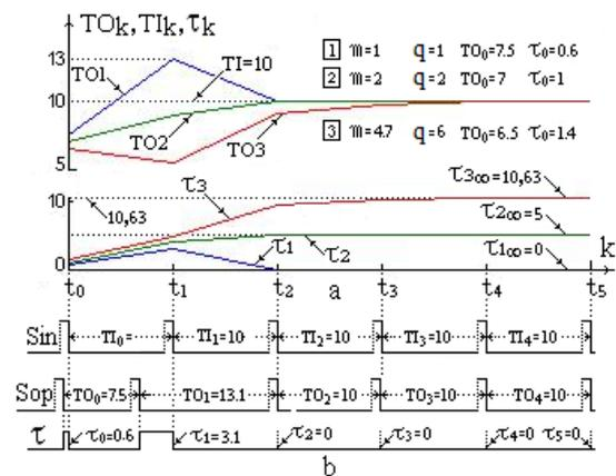
Fig. 7. (a). The output period tends to the input period and the final value of time difference  $\tau_\infty = TI(q-1)/m$ . (b). All periods of  $S_{in}$ ,  $S_{op}$  and time differences  $\tau_k$ , for the case Nr. 1, are calculated and presented to show the real time relation between variables. For this case,  $m=1$  and  $q=1$  ( $\tau_\infty=0$ ) and the circuit functions as a classic PLL.
