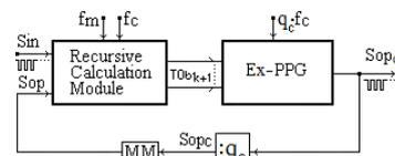
Fig. 5. The simplified principal scheme of the multiplier with Ex-PPG and a counter in the feedback connection. The multiplication factor is  $q_c$ .
