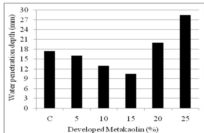
Fig. 2. Water penetration of ordinary and metakaolin concrete
