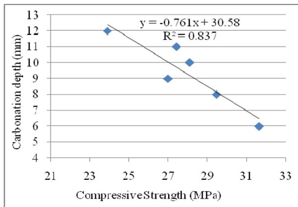
Fig. 7. Relationship of compressive strength and carbonation depth of metakaolin concrete
