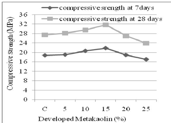
Fig. 1. Compressive strength of plain (C) and Metakaolin concrete
