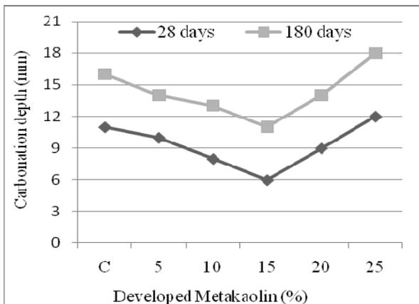
Fig. 4. Carbonation depth of ordinary and metakaolin concrete
