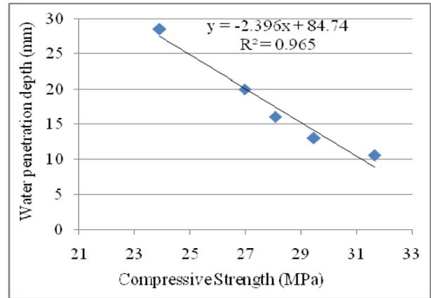
Fig. 5. Relationship of compressive strength and corrosion of metakaolin concrete
