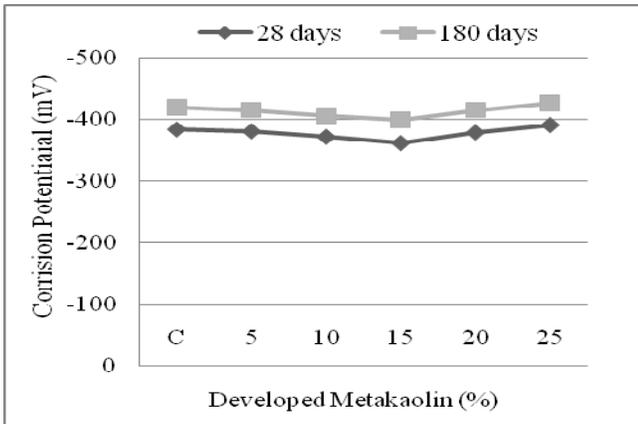
Fig. 3. Corrosion potential of ordinary and metakaolin concrete
