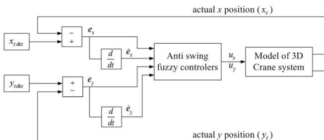
Fig. 4. Simulation block diagram of the 3D crane control.
