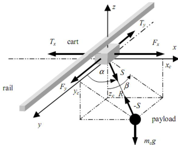
Fig. 2. 3D crane system: coordinates and forces.
