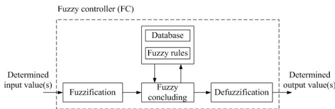
Fig. 3. Standard structure of fuzzy controller.
