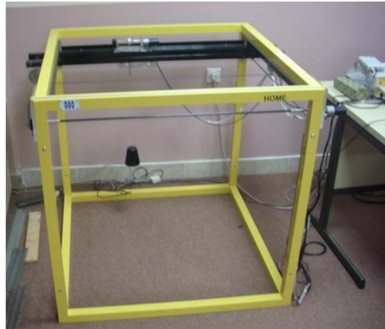
Fig. 1. 3D Crane System made by Inteco.
