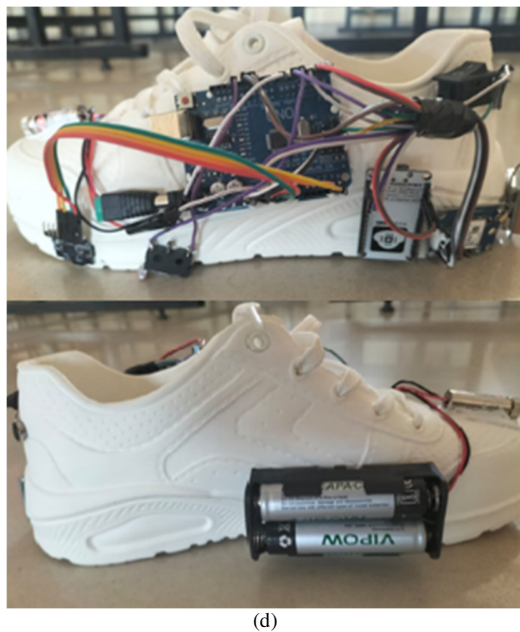
Fig. 6. Prototype of the assistive footwear system: (a) top view, (b) rear view, (c) laser projection, (d) side views of the prototype.
