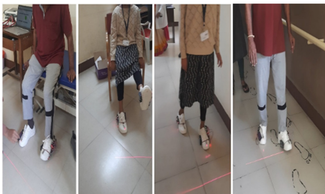
Fig. 7. Clinical validation at JSS PMR department, showing participants performing walking tasks with floor markings for standardized gait trials, sit-to-stand, and turning tasks while wearing the assistive footwear prototype.
