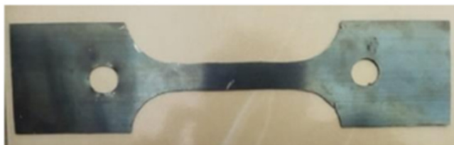
Fig. 4. Schematic and photograph of ASTM E8 pin-loaded specimen.
