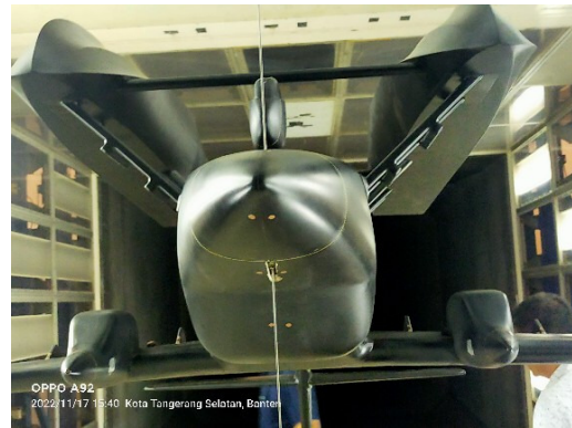
Fig. 2. Aerodynamic model of seaplane during wind tunnel test.
