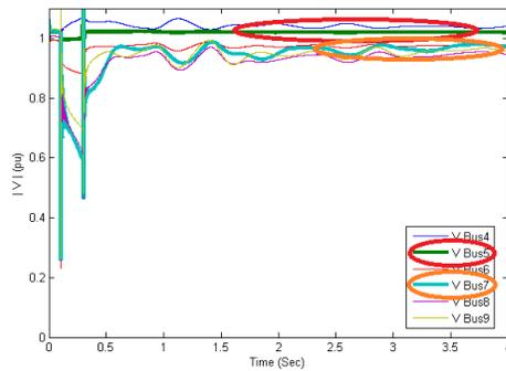
Fig. 12. The buses voltage in the presence of three-phase short circuit fault according to time (with STATCOM).
