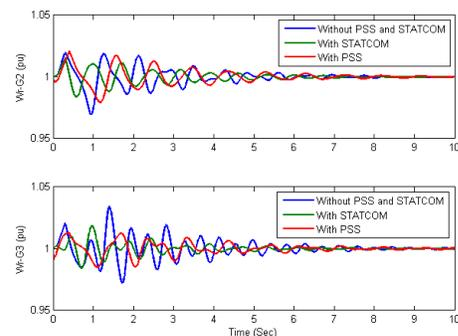
Fig. 15. Rotor angular velocity of generator (2) and (3) in the presence of three-phase short circuit fault according to time (based on optimized PD controller for PSS).
