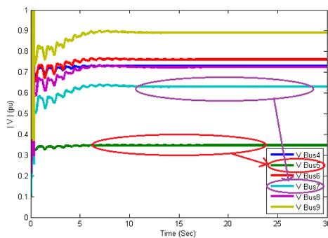
Fig. 14. The buses voltage in the presence of three-phase short circuit fault according to time (based on optimized PD controller for PSS).
