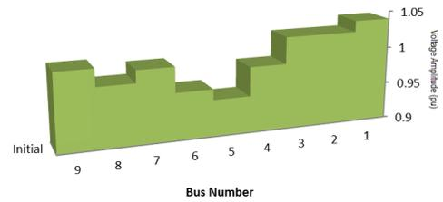
Fig. 4. Voltage buses in the initial state (without PSS and STATCOM)
