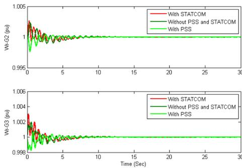
Fig. 9. The angular velocity of generators 2 and 3 according to time.
