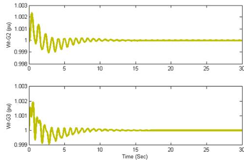
Fig. 5. Angular velocity of generators 2 and 3 according to time (without PSS and STATCOM and the controller)
