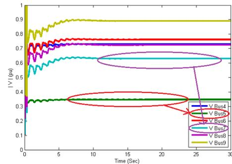
Fig. 10. The buses voltage in the presence of three-phase short circuit fault according to time (without PSS and STATCOM).
