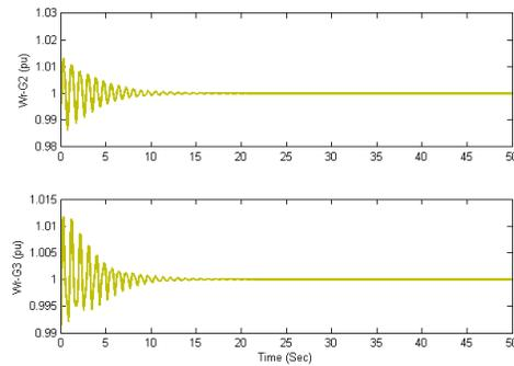
Fig. 11. Rotor angular velocity of generator (2) and (3) in the presence of three-phase short circuit fault according to time (without PSS and STATCOM).
