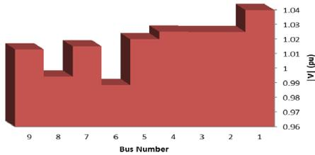
Fig. 8. The voltage buses with the presence of PSS
