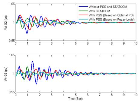
Fig. 16. Rotor angular velocity of generator (2) and (3) in the presence of three-phase short circuit fault according to time (based on optimized PD controller for PSS).
