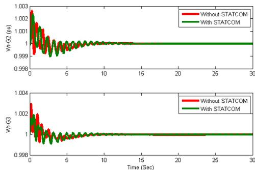
Fig. 7. Angular velocity of generators 2 and 3 with STATCOM (without controller).
