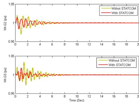
Fig. 13. Rotor angular velocity of generator (2) and(3) in the presence of three-phase short circuit fault according to time (with STATCOM).
