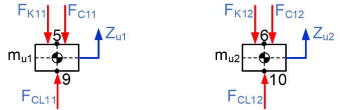
Fig. 3. Force model acting on the front axle (front view).
