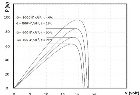
Fig. 4. P-V curve of PV cell without MPPT.
