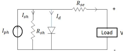
Fig. 2. Equivalent circuit of a PV cell.
