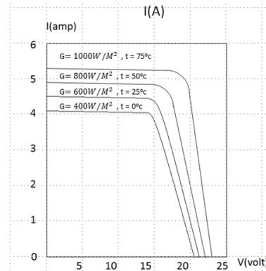
Fig. 3. I-V curve of a PV cell without MPPT.
