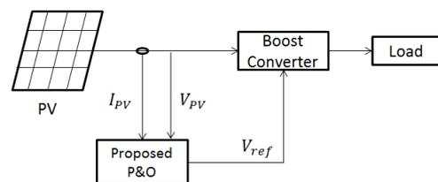
Fig. 1. Block diagram of the P&O method.
