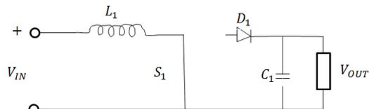
Fig. 6. Boost Converter Operation at Switch ON.
