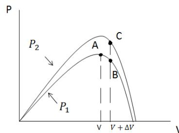
Fig. 9. Separation diagram of MPP for P&O.
