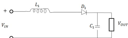
Fig. 7. Boost Converter Operation at Switch OFF.
