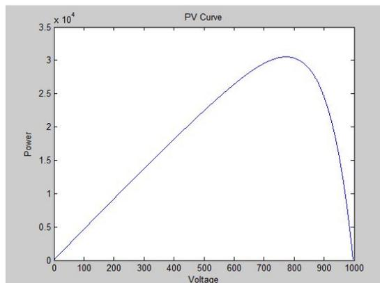
Fig. 10. PV curve of P&O MPPT.
