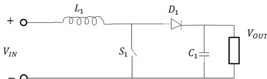
Fig. 5. Basic Boost Converter Circuit.
