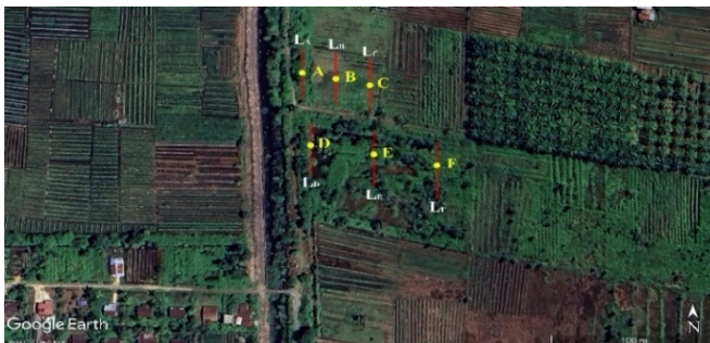
Fig. 2. Geophysical measurement positions using the Wenner configuration of the geoelectrical method.
