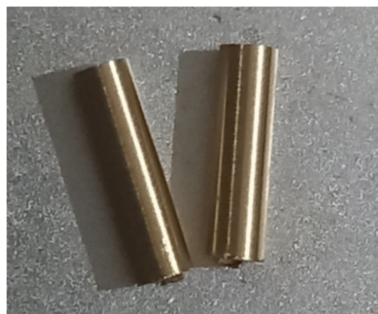
Fig. 1. MMC specimen for pin-on-disc tests.
