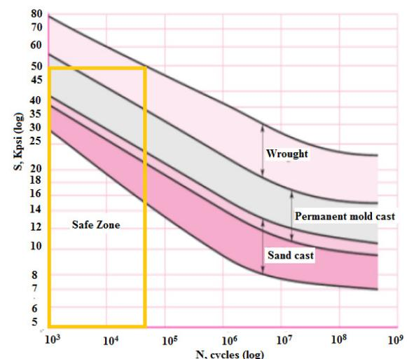
Fig. 3. The safe zone for blood bank centrifuge's bucket.
