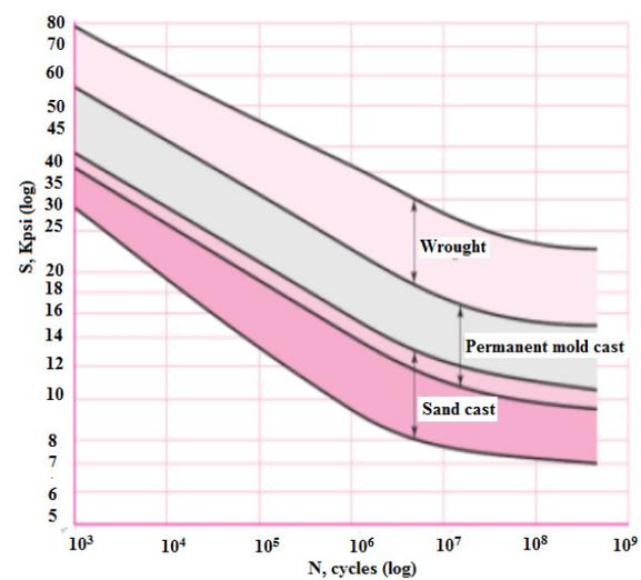
Fig. 2. S-N diagram for aluminum alloys
