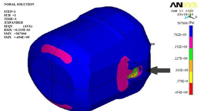
Fig. 1. The FEM results of the stress contours occurred in a bucket during centrifuge process.
