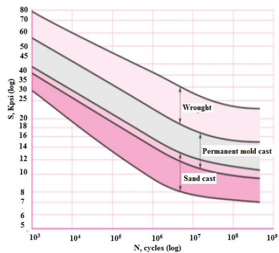
Fig. 2. S-N diagram for aluminum alloys
