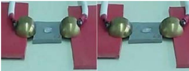
Fig. 3. Deformation of a single droplet on sample A (droplet conductivity 1.4  $\mu\text{S}/\text{cm}$ )
