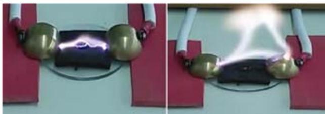
Fig. 4. Arcing of a single droplet on sample C
