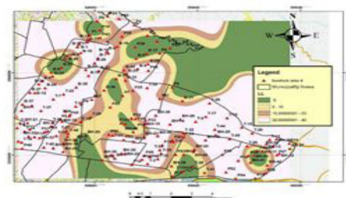
Fig. 5. The Atterberg limits zoning map at a depth of 10 meters of Zone 4
