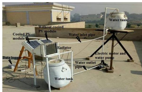
Fig. 1. Fabricated active cooling system.
