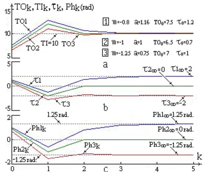
Fig. 3. Phase shifting ( $T=0$  for all of three cases) in the function of parameters "m" and "a": a. The output period tends to the input period, b. The final value of time difference  $\tau_{\infty} = TI(1-a)/m$ , c. The final value of the phase shifting is  $Ph_{\infty} = 2\pi \cdot \tau_{\infty} / TO_{\infty}$  [rad] =  $2\pi(1-a)/m$  [rad].
