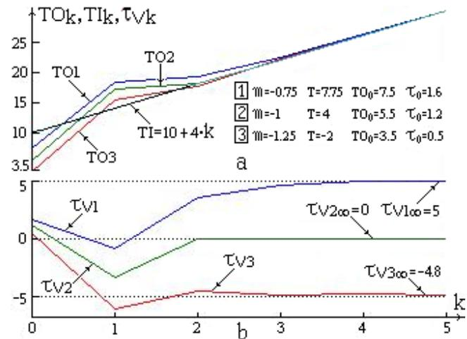
Fig. 4. The time shifting of the ramp input function ( $a=1$ ): a. The output periods, for all of three cases, track the input periods without an error,  $K_V=0$ , b. The time shiftings tend to the time differences  $\tau_{V\infty}$ , given by eq. (14).
