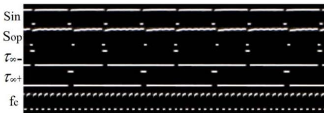
Fig. 6. The shifter is in the stable state. It functions as PLL ( $a=1$ ,  $m=-1$ ,  $T=0$ ). The ratio  $TI/t_c$  is only about six and the time differences  $\tau_{\infty+}$  and  $\tau_{\infty-}$  are visible. If  $TI/t_c$  increases, the time differences tend to zero.
