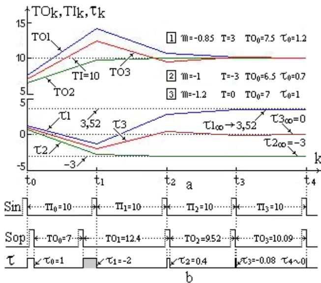
Fig. 2. Time shifting ( $a=1$  for all of three cases): a. The output period tends to the input period and the final value of time difference  $\tau_{\infty} = -T/m$ , b. The case Nr. 3, in Figure 2a, is presented in the real time form. All periods of Sin, Sop and time differences  $\tau_k$  are calculated, showing the real time relation between them. For this case,  $T=0$  ( $\tau_{\infty}=0$ ) and the shifter functions as a classic PLL.
