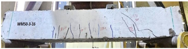
Fig. 14. Final crack pattern of specimen WM50-3-16.
