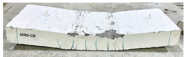
Fig. 19. Crack pattern of specimen WR0-CB.
