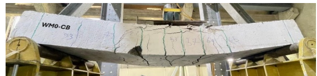
Fig. 8. Final crack pattern of specimen WM0-CB.
