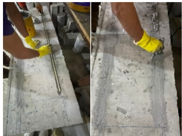
Fig. 5. Strengthening using GFRP bars.
