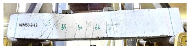
Fig. 12. Final crack pattern of specimen WM50-2-12.
