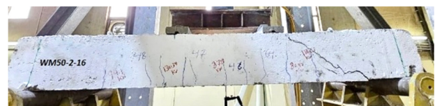
Fig. 13. Final crack pattern of specimen WM50-2-16.
