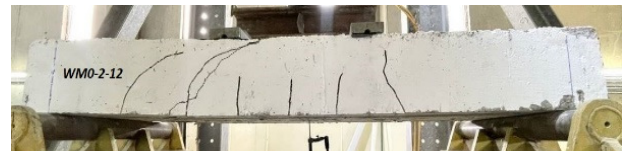
Fig. 9. Final crack pattern of specimen WM0-2-12.
