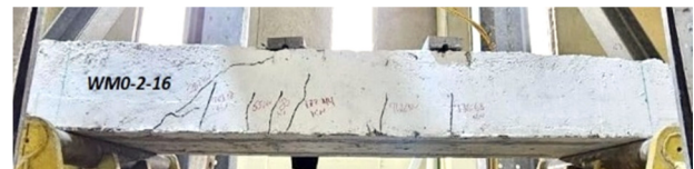
Fig. 10. Final crack pattern of specimen WM0-2-16.
