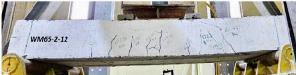
Fig. 15. Final crack pattern of specimen WM65-2-12.
