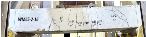
Fig. 16. Final crack pattern of specimen WM65-2-16.
