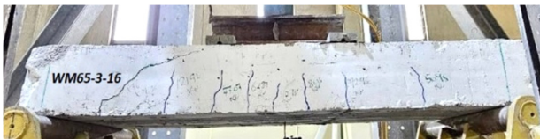
Fig. 17. Final cracks pattern of specimen WM65-3-16.
