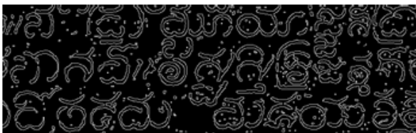
Fig. 10. Canny edge detection image of a low-noise stone inscription.
