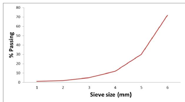
Fig. 2. Grain Size Distribution Curve of Waste Tile Fine Aggregates
