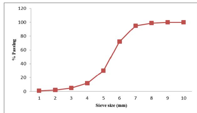
Fig. 1. Grain Size Distribution Curve of Waste Tile Coarse Aggregates.
