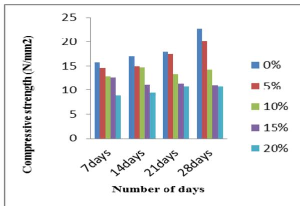
Fig. 3. Compressive Strength of Concrete with Waste Tiles as Fine Aggregates
