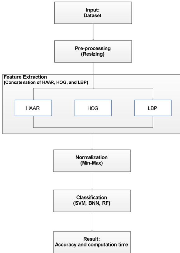
Fig. 5. Proposed system for classification of moving objects on the road and classification of motorcyclists wearing helmets.
