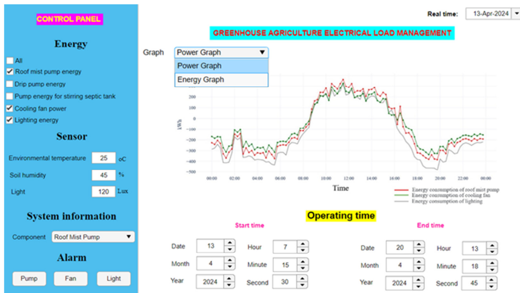
Fig. 7. System for monitoring energy consumption and environmental parameters.
