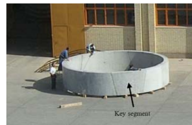
Fig. 1. Assembled ring in segment manufacturing factory, Tabriz metro-Line 1
